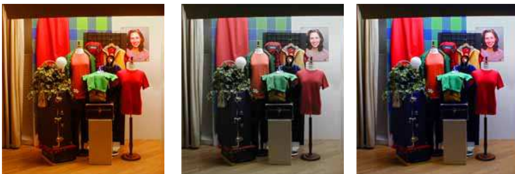
Figure 36. Same picture, with an incandescent bulb (left), GE cool white bulb (middle), and GE Chroma 50 (right).
